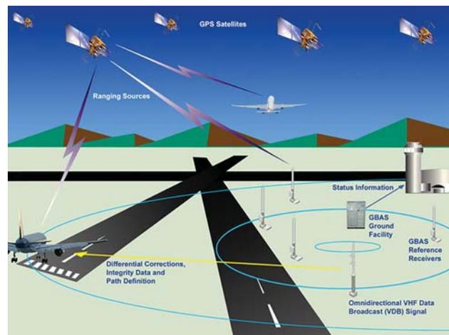
Figure 1. Example of a Ground-based Augmentation System (Source: United States Federal Aviation Administration)
